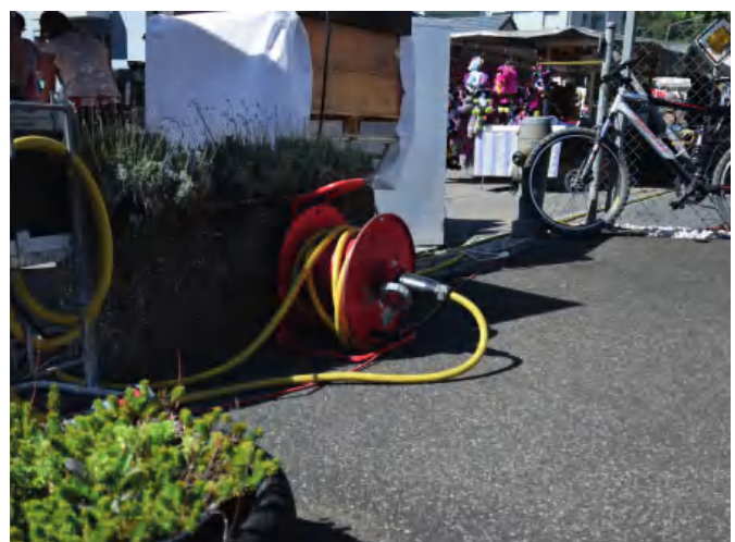
Cable reel with a metal body
